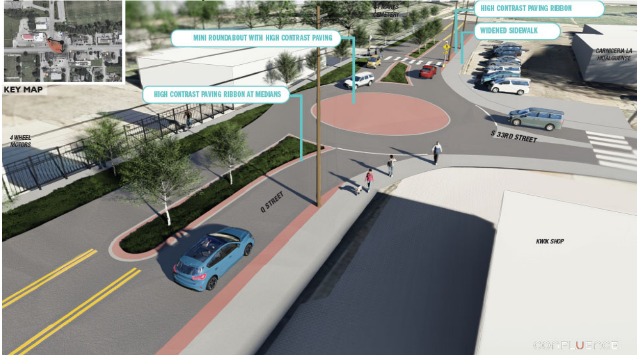
Figure 6-5. Q Street Conceptual Alternatives I-B with Roundabout Intersections
