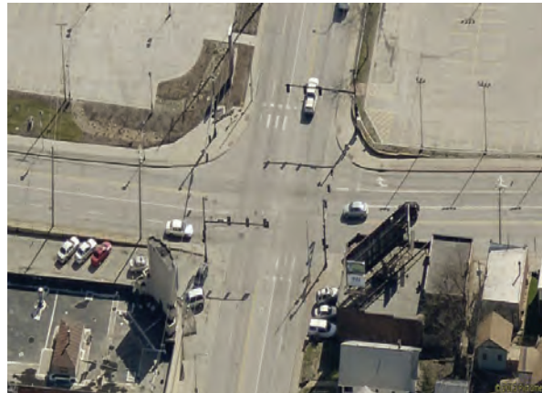
Figure 19: Intersection with lack of physical pedestrian cues.
