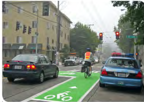
Bike boxes and green pavement (combined in this example) are two tools for improving intersections for bicyclists.
