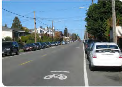
The placement of Shared Lane Markings varies based on lane width and the presence of on-street parking.
