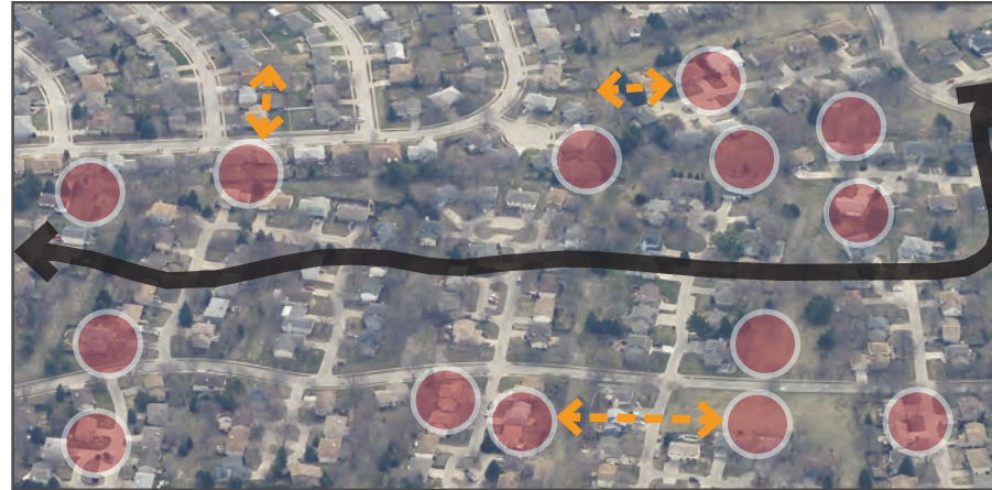
Figure 6: Cul-de-sacs Prevent Neighborhood Connections and Channelize Traffic to a Single Street (photo base images accessed from Pictometry Online)
