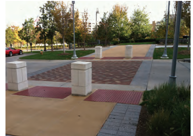
Figure 11: Consistent walkway through amenity zone (left). Specialty paving outside of walkway (right).
