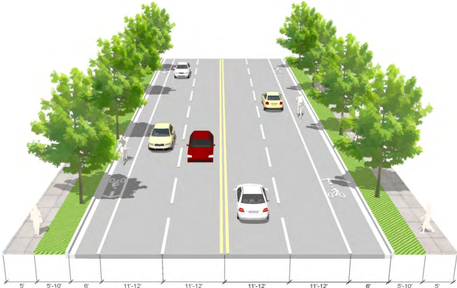
Figure 2: Four lanes with bike lanes and sidewalks, no parking
