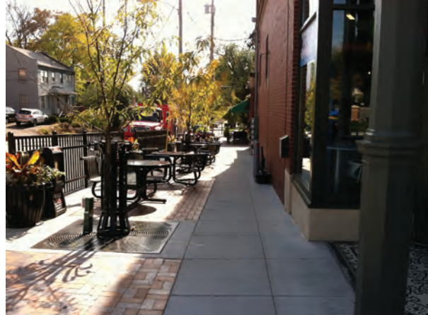
Figure 11: Consistent walkway through amenity zone (left). Specialty paving outside of walkway (right).
