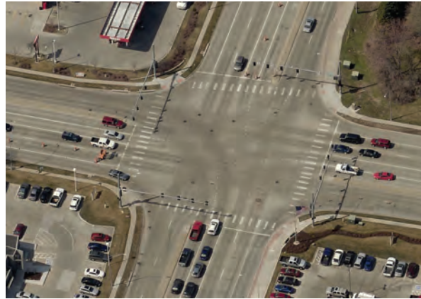
Figure 18: Intersection with excessively wide streets (left). Long distance required to cross the wide street (right).
