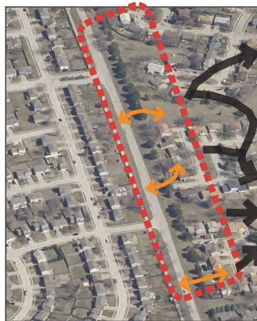
Figure 7: Too Few Entry-and-Exit Points Create Congestion Issues because of Limited Routing Options (photo base images accessed from Pictometry Online)
