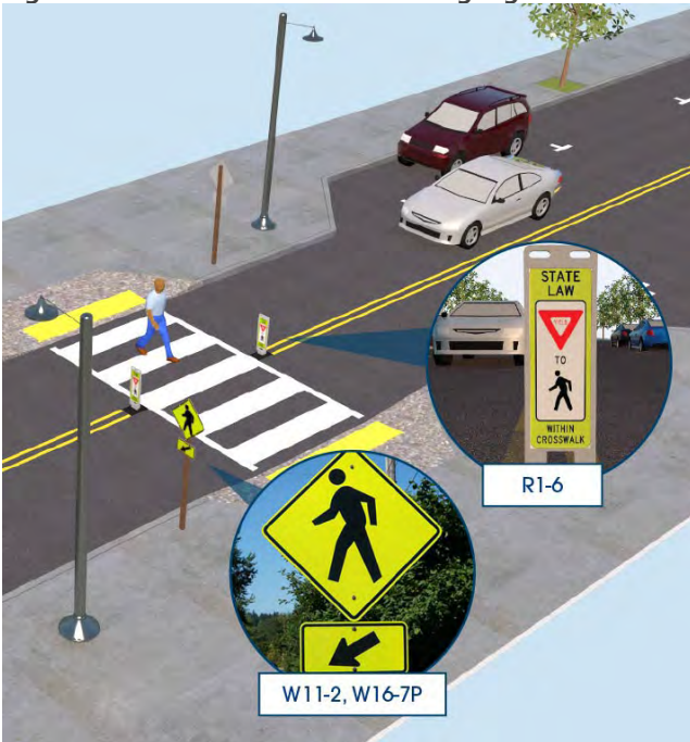
Figure 6: Midblock Crosswalk with Signage
