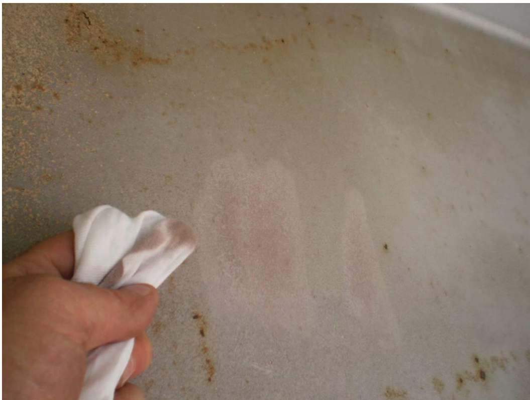
Photograph 3 – Span 5 – Finish Coat could be Removed by Rubbing with a Soft Cloth
